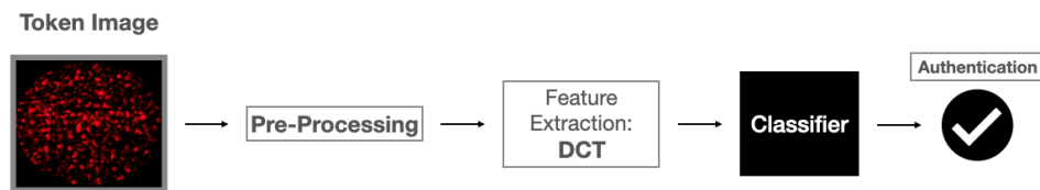
Figure 4.13: Authentication Phase - Approach 2: Pipeline for the authentication of tokens against other registered tokens in a database utilizing the DCT and a Classifier.
