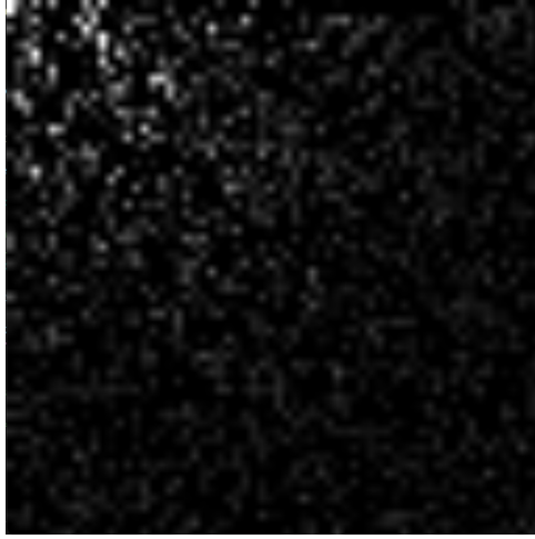
Figure 4.9: Example of a DCT matrix obtained from a 64x64 resized speckle pattern. Most of the energy tends to be compacted in the first coefficients of the matrix, i.e. the upper left corner.
