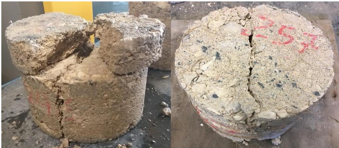
Figure 10 - Comparison between the final state of specimens without CF (left) and with CF (right)
