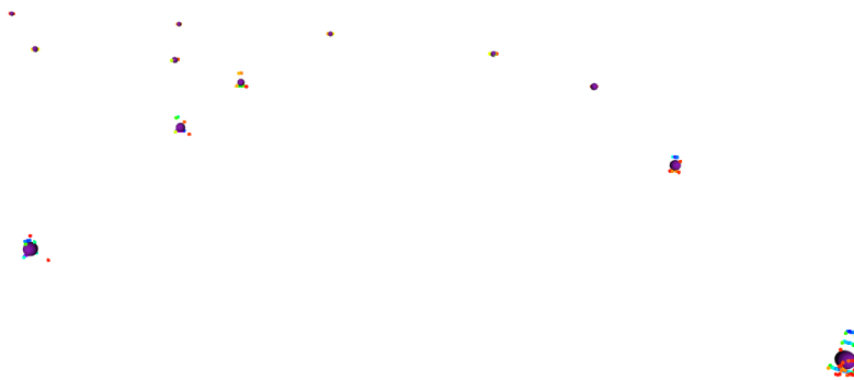
Figure 4.4: Result of the Euclidean clustering method applied to the filtered point cloud shown in Fig. 4.3(b). Each purple sphere represents the 3D centroid of its corresponding cluster, identifying the different clusters.
