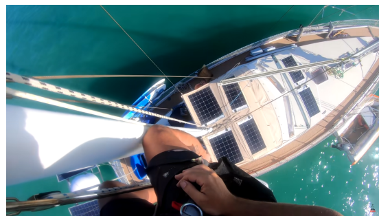
Figure 10: SV Delos - Center mounted flexible 2 170W and 4 110 W panels.
