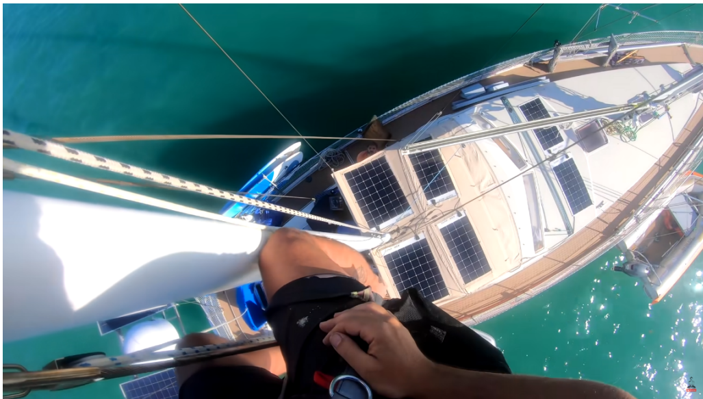
Figure 5.3: SV Delos - Center mounted flexible 2 170W and 4 110 W panels.
