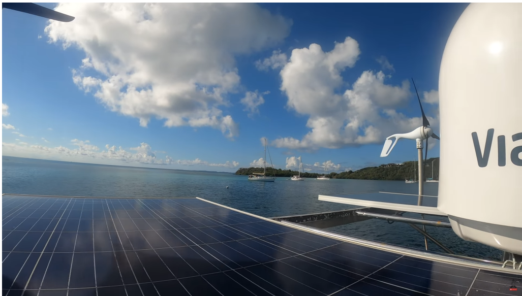
Figure 5.2: SV Delos - Turbines and rear mounted 2 X 330W Canadian Solar panels.
