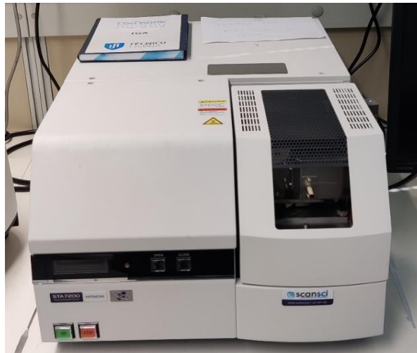
Figure 15. Model 7200 Simultaneous Thermal Analyzer.
