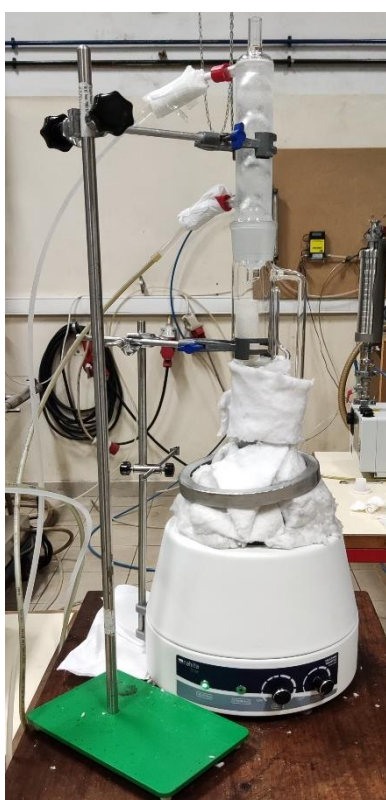
Figure 13. Setup for extractive determination.
