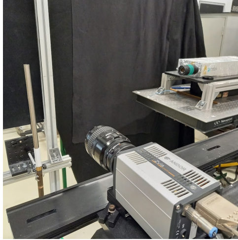
Figure 2.4: Experimental setup for the PIV experiments. Camera on the center, laser on the top right of the picture and Bunsen tube on the left.
