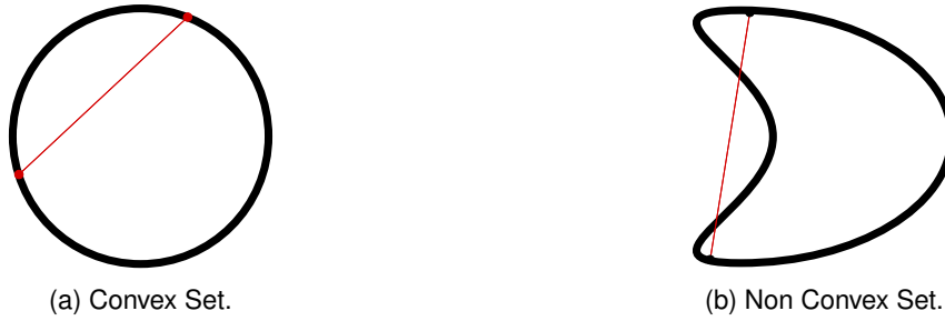
Figure 2.8: Illustration of a convex set. A set C is convex if the line segment between any two points in C lies in C . All convex sets must verify the condition: if x_1, x_2 \in C then tx_1 + (1-t)x_2 \in C with 0 \leq t \leq 1 (Adapted from [24]).
