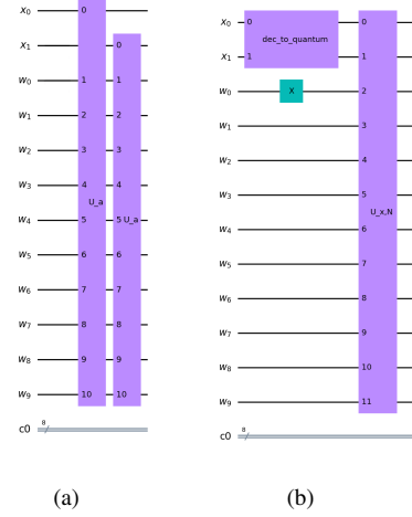
Fig. 7. Quantum circuits for the U_{x,N} gate. (a) Quantum circuit to implement the U_{x,N} gate; (b) Quantum circuit to test the U_{x,N} gate;
