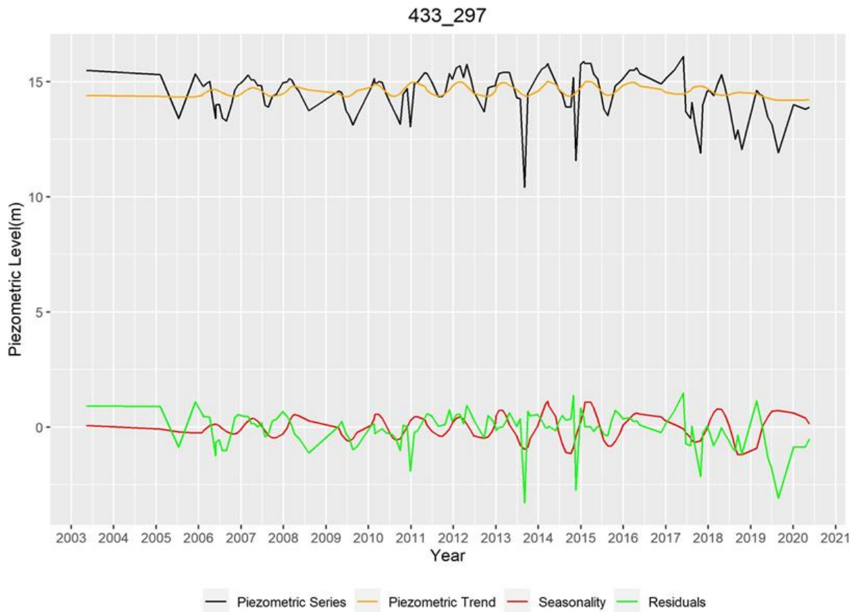
Figure 4.40: The figure showing the groundwater level trend, seasonality, and residuals of well 433/297
