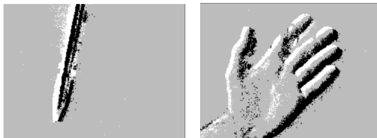
Figure 1.2: Outputs of event cameras under various situations, a pen moving in front of the camera (left), and a person’s hand waving in front of the camera (right). White and black denote the polarity of the event being represented, in particular positive and negative, respectively.
