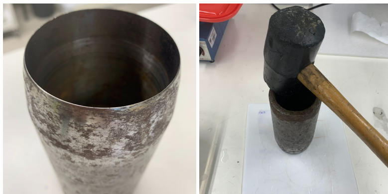
Figure 3.7: Membrane cutting step. Metallic cutting circular impression is visible on the left-side.
