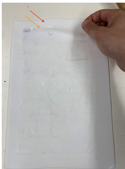
Figure 3.6: Membrane hybrid flat-sheet disposition for cutting
