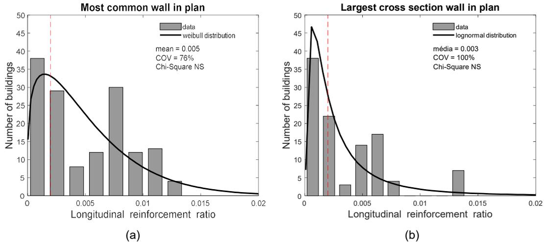
Figure 4 - Longitudinal reinforcement ratio for the (a) most common shear wall and (b) largest cross-section shear wall in plan
