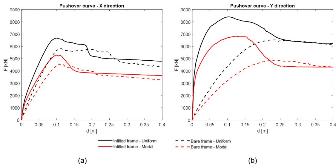
Figure 6 - Pushover curves for the bare and infilled frame models considering both lateral load types and for the (a) X and (b) Y direction
