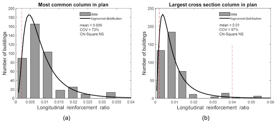
Figure 3 - Longitudinal reinforcement ratio for the (a) most common column and (b) largest cross-section column in a plan
