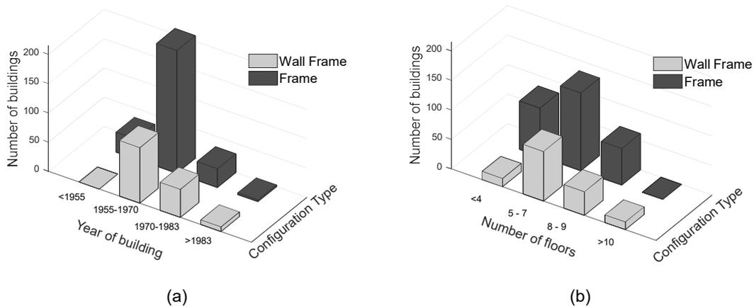
Figure 2 - Results of the data collected from the buildings in Benfica, in function of the (a) construction period vs type of configuration and (b) the number of storeys vs type of configuration.
