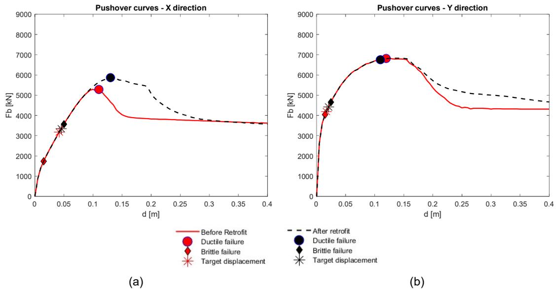
Figure 7 - Pushover curves with the indication of the target displacement and the failure displacements for the constraining action before and after retrofitting solution for (a) X and (b) Y direction
