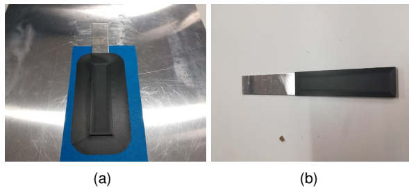
Figure 1: (a) Nylon CF15 specimen's resting time after printing and (b) after removal of the brim.
