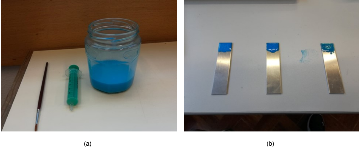
Figure 3.10: (a) ABS primer's application tools and (b) three examples of base material with primer applied.
