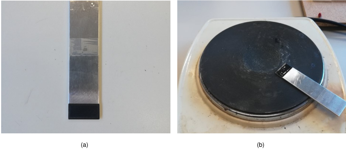
Figure 3.13: (a) Nylon CF15 specimen's coating printing and (b) remelting on top of a hot plate.
