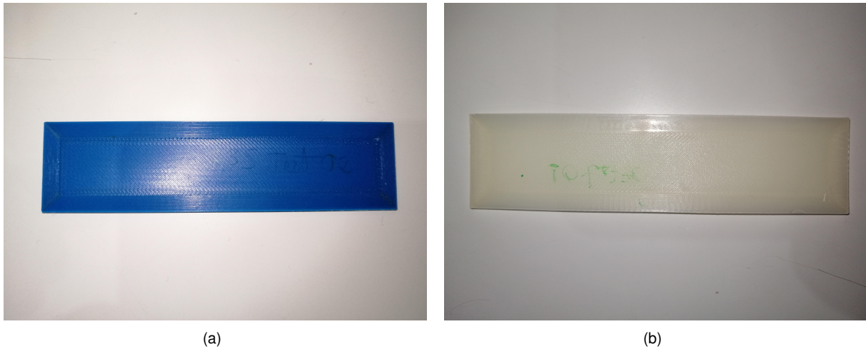
Figure 3.5: (a) ABS and (b) Nylon top adherend printing's calibration.
