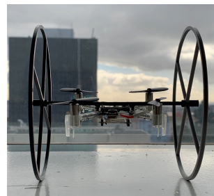
Figure 1: Prototype of the Bimodal aerial robot, consisting of a quadrotor with two passive wheels.
