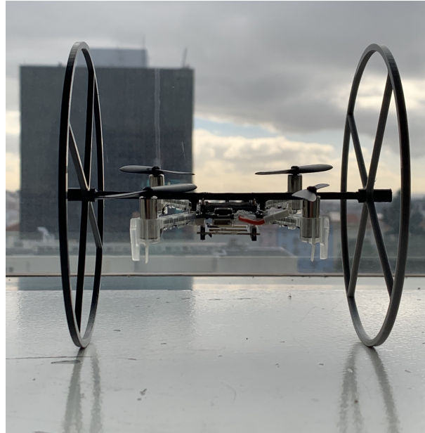
Figure 1.1: Prototype of the Bimodal aerial robot
