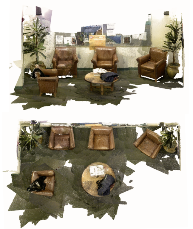
Figure 9: Reconstruction of the Lounge dataset [23] with 3000 poses. PGO computed by EigenMA in 0.15s.
