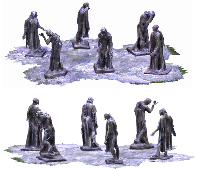
Figure 8: Reconstruction of the Burghers dataset [23] with 1124 poses. PGO computed by EigenMA in 0.04s.
