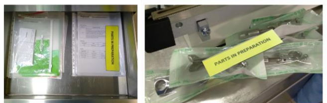
Figure 7 – Work pass identification card between shifts
