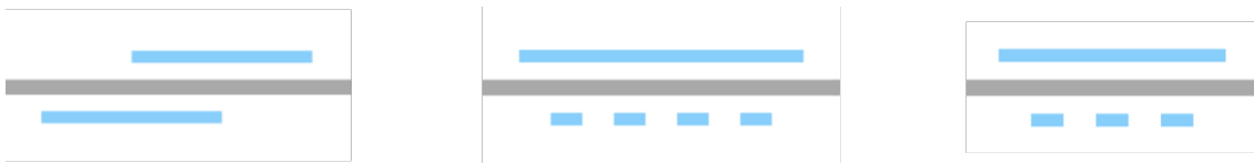
Figure 5.7: Group station (left), Base position (middle) and Charging station (right) markers
