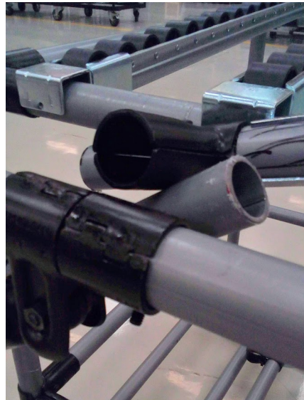
Figure 4.9: Simple stopper aperture problem
