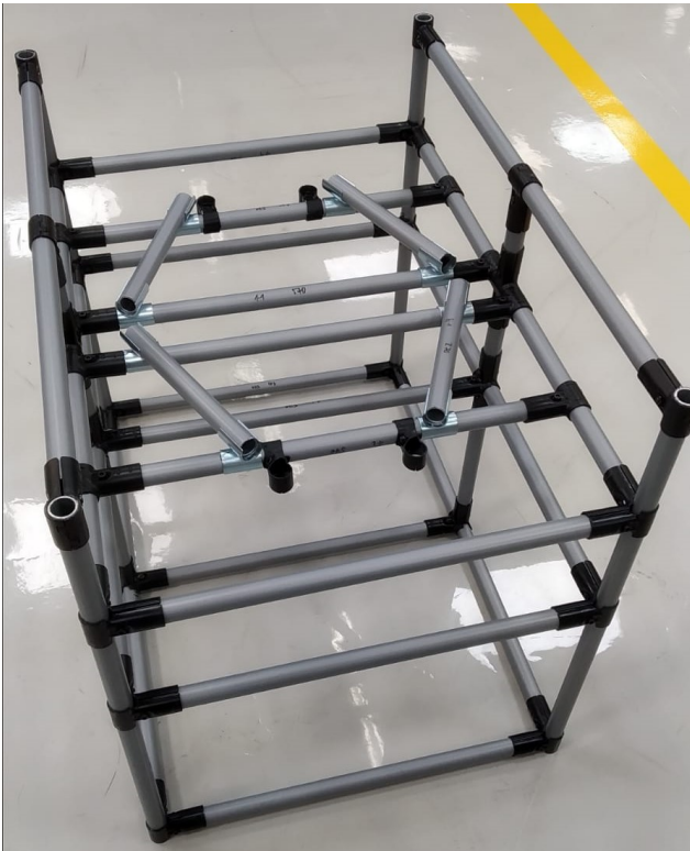
Figure 4.2: Picture of the cart during the assembly, coupling structure shown
