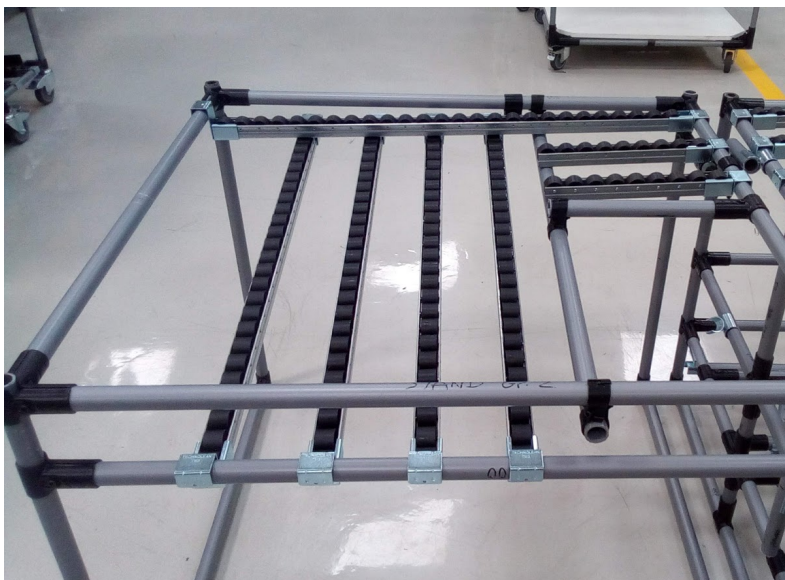
Figure 4.19: First non-working version of the group stand
