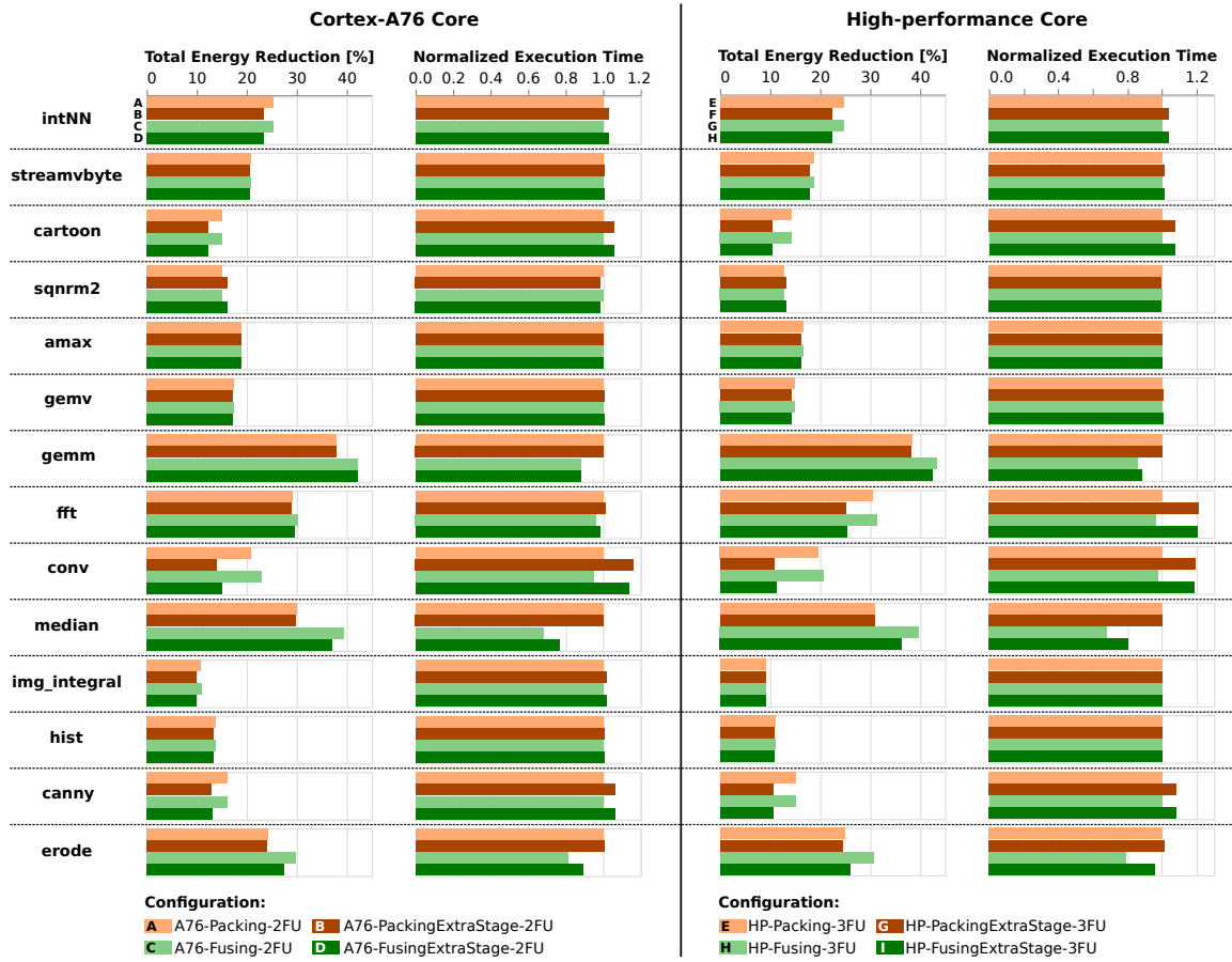
Figure 6.5: Impact of adding a new pipeline stage in the vector unit in terms of the total energy reduction and normalized execution time, for the packing and fusing modes, and the Cortex-A76 and High-performance cores.
