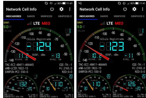
Figure 19 - Measurements performed in an indoor environment with the mobile terminal connected to the eNB 1822.
