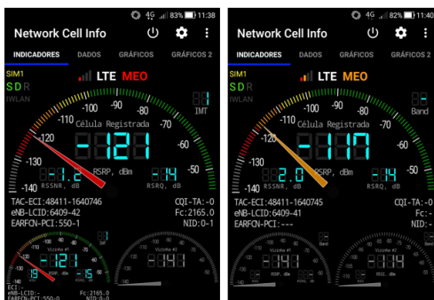
Figure 18 - Measurements performed in an indoor environment with the mobile terminal connected to the eNB 6409.
