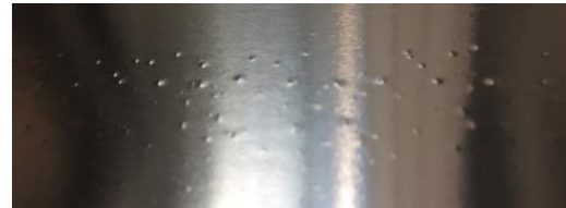
Figure 16: Indentations on the Al surface due to 1100 rpm operation
