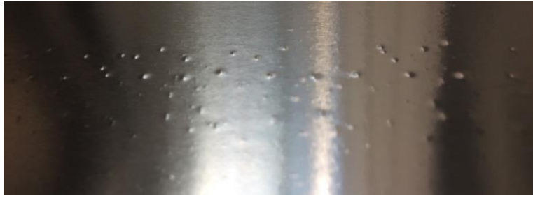
Figure 4.16: Indentations on the Aluminum surface after high-speed operation
