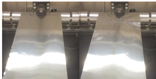
Figure 4.14: Behavior of the partially baggy web
