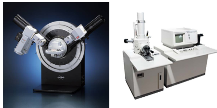
Figure 2.7: Equipments used for the physico-chemical characterization of the synthesized samples. Left: Bruker AXS-D8 Advance powder diffractometer. Right: Scanning Electron Microscope Hitachi S2400.
