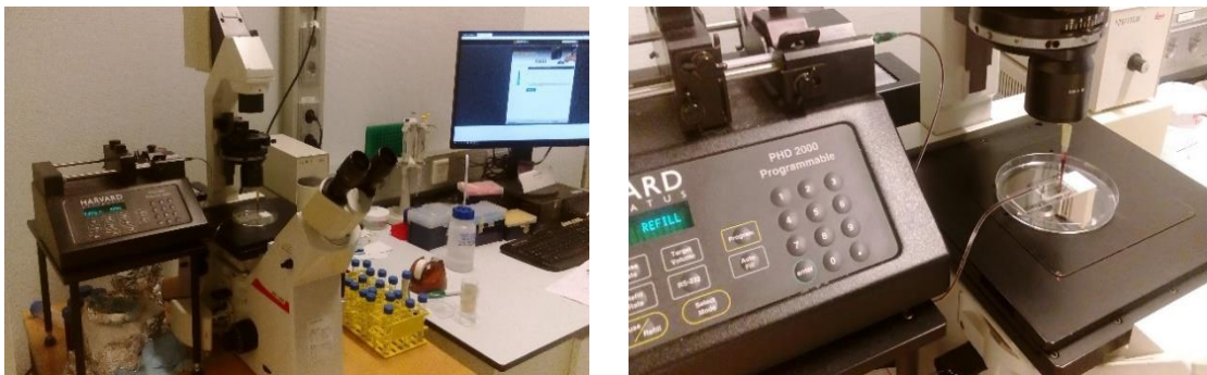
Figure 20 – Pictures of the setup used for blood perfusion experiments. The microchip was placed inside a Petri dish on top of the microscope platform. The outlet was connected to a syringe placed on the pump. A pipette tip filled with blood was introduced in the inlet and the blood was pulled by the pump through the channel. A side camera connecting the microscope and the computer allowed for real-time record of the experiment.
