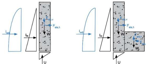
Figure 5.1 – Loads on the two models: static in black and dynamic in blue.
