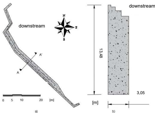
Figure 3.2 – Dam's plan and middle cross section.
