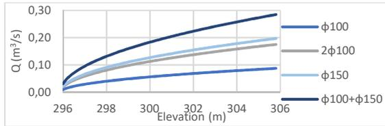
Graph 4.1 – Discharge curves for the hypothetical geometries of the outlets/ducts.
