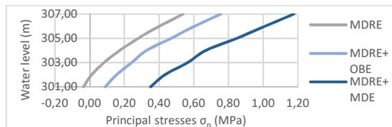
Graph 5.1 – Tensile stresses on the heel of the dam for the model with the dam and the building.
