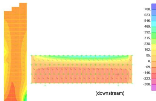
Figure 5.3 – Maximum stresses distribution for Dynamic-MDE scenario, for 303 m of water level (model with building).
