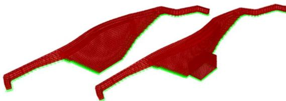
Figure 5.2 – First modal shapes for the gravity dam (left) and dam with the building (right).
