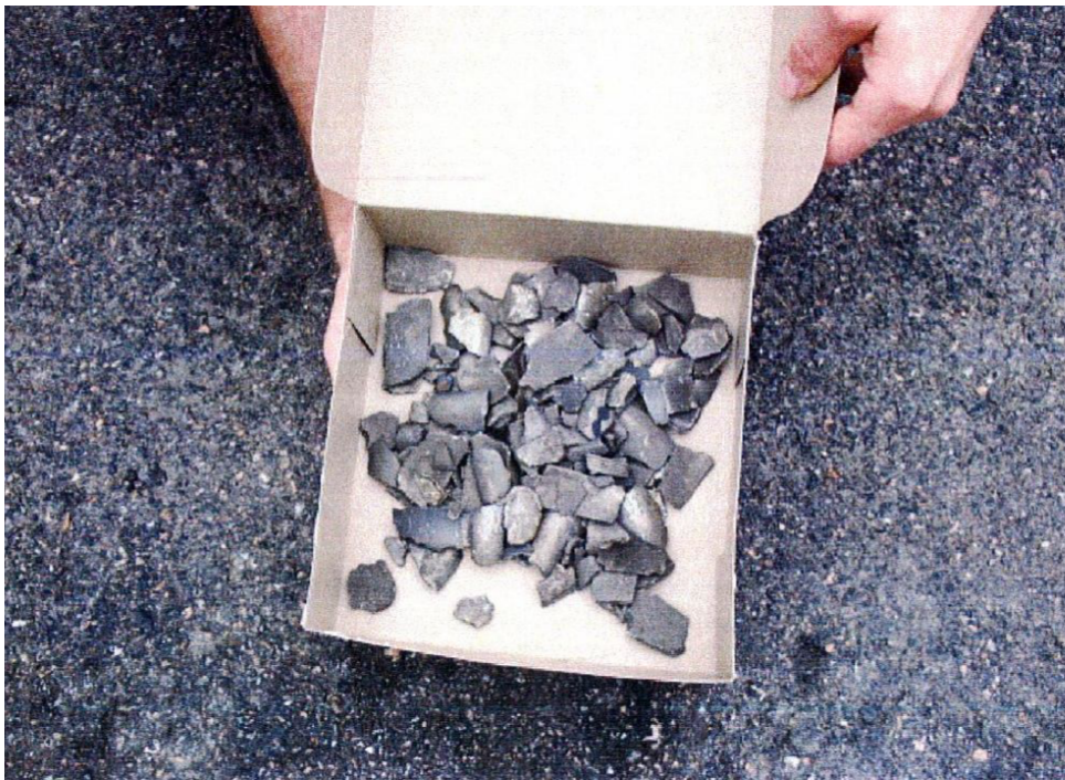
Figure 4.2: Pieces of engine found by the airport maintenance unit on runway 22R [51]
