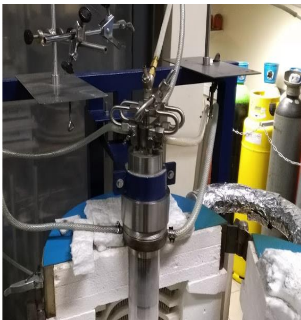
Figure 11: Injector with air and water supplies.
