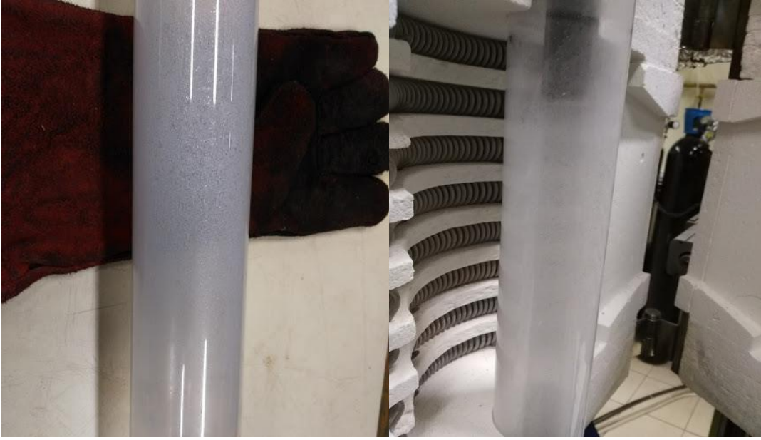
Figure 24: Damaged quartz tube.
