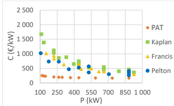
Figure 5 – Turbomachines' unit cost
