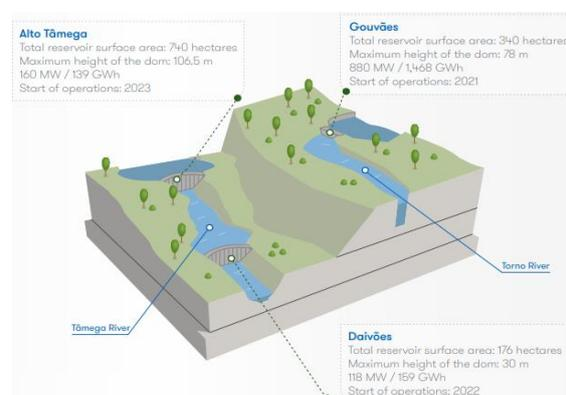
Figure 1 – Tâmega hydropower complex (Iberdrola 2017)
