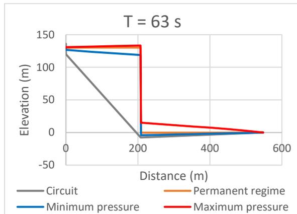
Figure 10 – Pressure variation along the circuit
