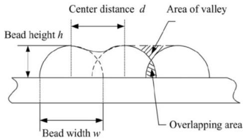
**Figure 3:** Overlapping welding beads illustration for parallel and oscillation strategies [50].
