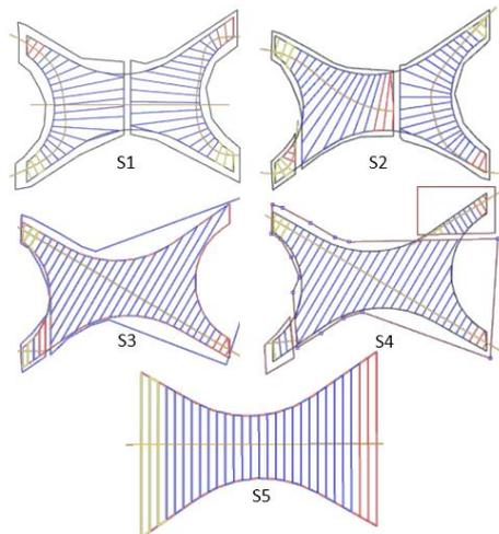
**Figure 4 :** Deposition strategies considered (S1-S5), numbered by deposition order of the sections.
