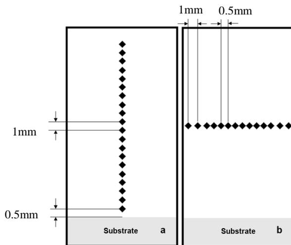
**Figure 6 :** Hardness test points. a) Vertical measurements and b) horizontal measurements. Figure not to scale.
