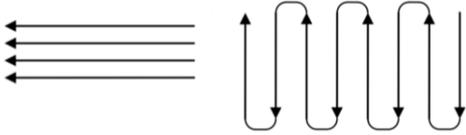
**Figure 1:** Deposition path strategies. (a) Parallel wall and (b) Oscillated wall strategy [46].
