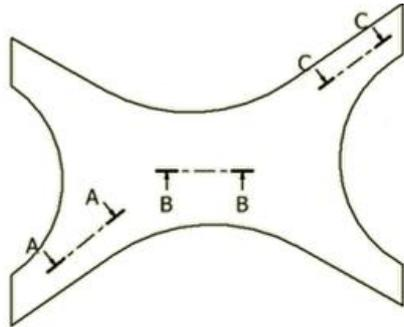
**Figure 5 :** Cut sections for the different deposition strategies. (a) For the strategies 1-4. For S5 the cuts were made in the same areas.
