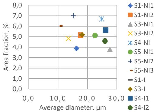
**Graph 1:** Pore area fraction by average pore diameter on the analysed sections.
