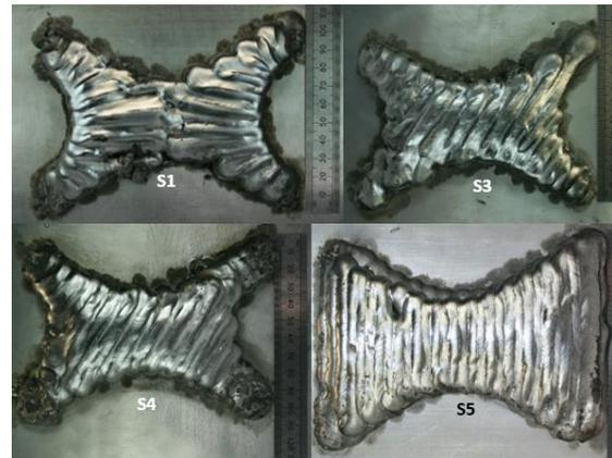
**Figure 7 :** Deposited parts with AA2319 as feedstock and AA6082 as build plate.
