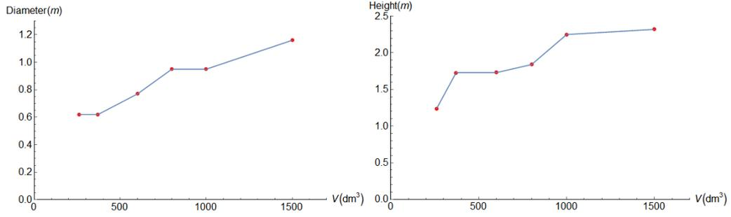
Figure 4: Linear interpolation of the tank's volume with its height and diameter
