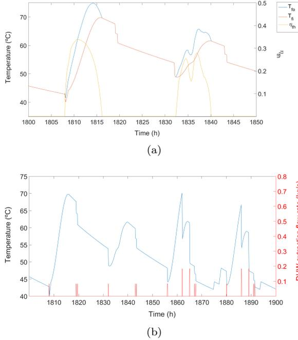
Figure 11: a) Detailed view, from the S1 optimization, of the entering,  $T_{fi}$ , and exiting,  $T_{fo}$ , water temperatures (left  $yy$  axis) and thermal efficiency,  $\eta_{th}$  (right  $yy$  axis), of the PVT array, b) detailed view for a specific DHW weekly consumption comparing  $T_{DHW}$  (left  $yy$  axis) with the DHW extraction flow rate,  $\dot{m}_{extr}$ , (right  $yy$  axis).
