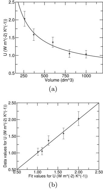
Figure 5: a) Fitting results of  $U_{IT} = V_{IT}^b + c$  with calculated  $U$  values and b) fit residuals from LAPESA Inertial Tank's data
