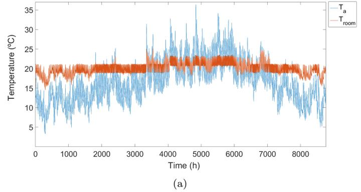
Figure 12: House room temperature,  $T_{room}$ , and ambient temperature,  $T_a$ , during a year from S1 optimization
