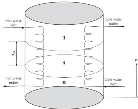
Figure 2: Inertial tank in thermal contact with the heat exchanger [19]
