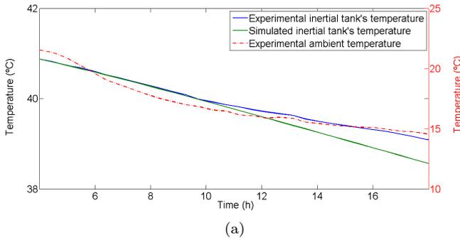
Figure 6: Simulink implementation of Inertial Tank heat transfer coefficient  $U_{IT}$  validation and b) its results in comparison with the tank's experimental change in temperature over time
