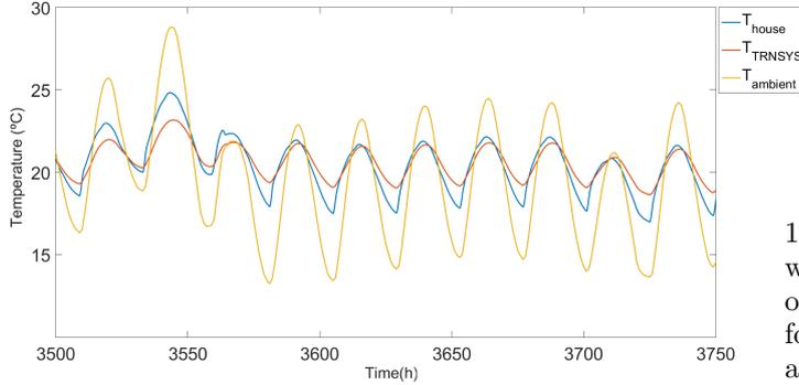
Figure 9: Detailed comparison of the house's room temperature change between the TRNSYS and SIMULINK implementation over a specific summertime period.
