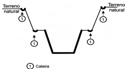
Figure 2- Surface drainage in canals (Rijo, 2010)
