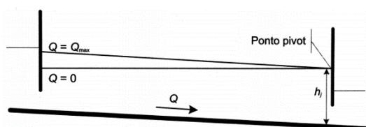
Figure 1- Water level control downstream the canal stretch (Rijo, 2010)
