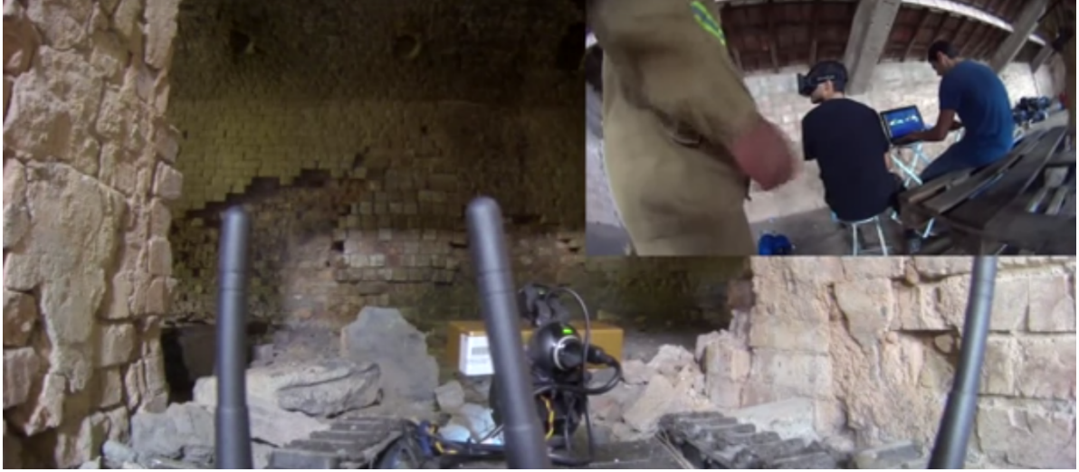
Figure 2.2: RAPOSA-NG during an on-field exercise. On the bottom, and teleoperation team, on the top-right, using the Oculus Rift and the teleoperation console [4].
