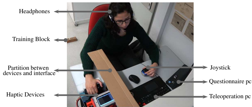
Figure 5.1: Teleoperation Station: participant using the joystick and the Traction Cylinder while receiving Visual feedback.
