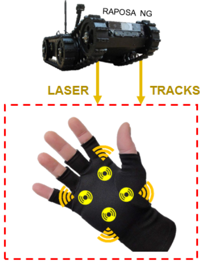
Figure 4.4: Concept Development: Vibrotactile Glove, where the yellow circles represent vibration actuators.
