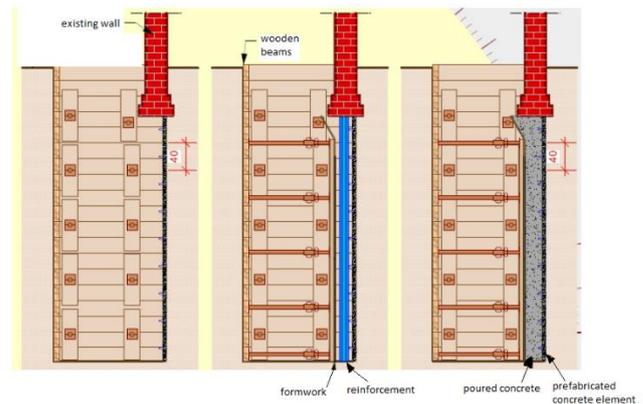
Figure 9: Underpinning in a contained slot
