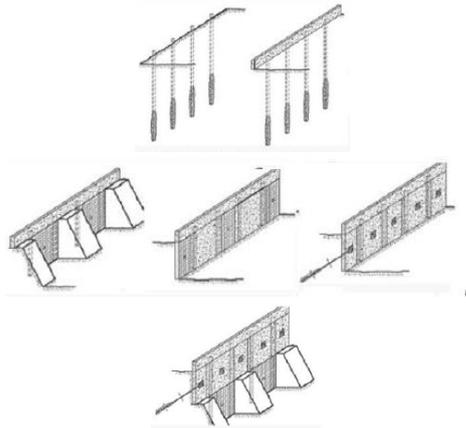
Figure 1: Munich type walls
