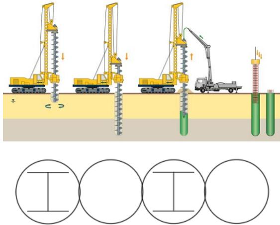
Figure 10: Mini CFA piles
