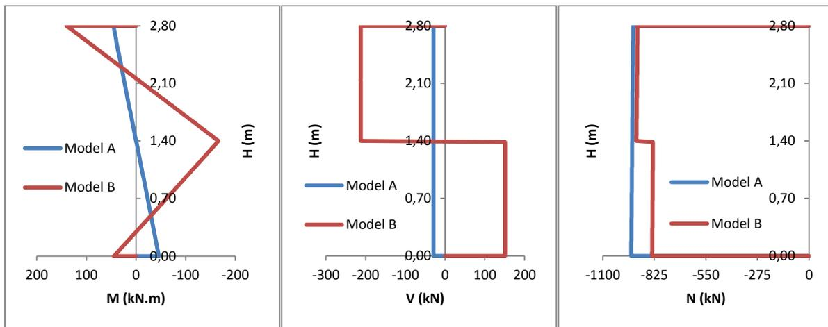
Figure 4 – Internal forces diagrams on the right column
