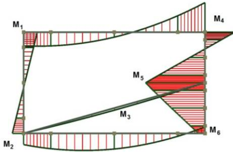
Figure 7 – Bending moment diagram (analyses Type II)
