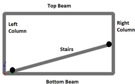
Figure 3 – Structural elements of Model B
