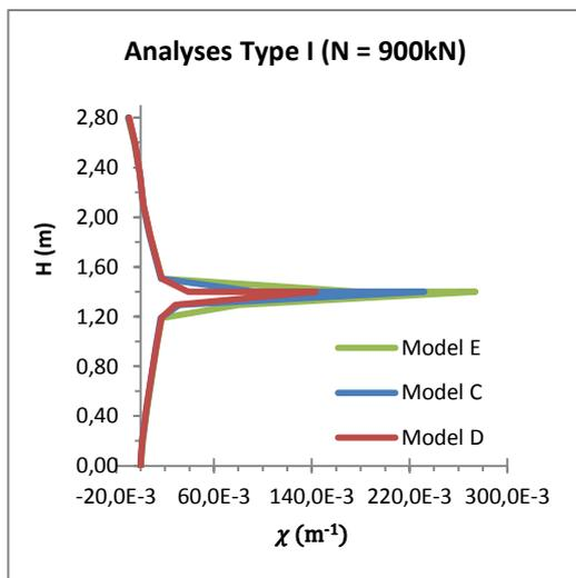
Figure 8 – Right column curvatures diagrams
