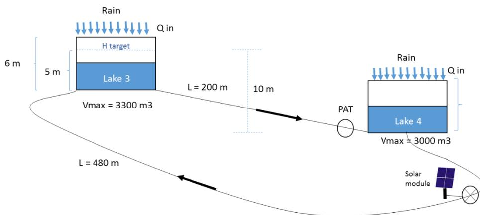
Figure 43 - Scheme of the SUDS technological solution implemented in the two decorative lakes in BCC (Low Region of BCC).
