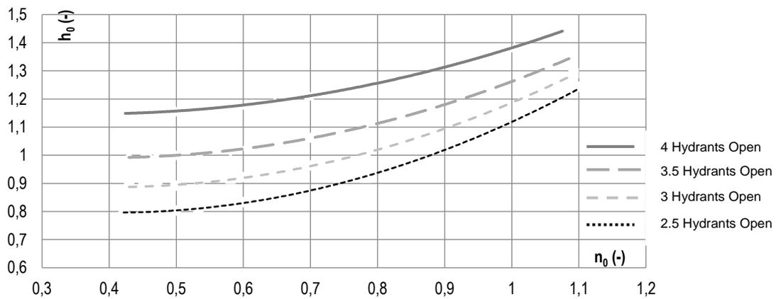
Figure 24 – Relative head by relative imposed nominal rotation
