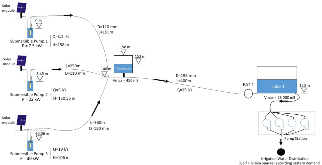
Figure 37 - Medium Region of BCC WDS - PAT 1 scenario schematic design.
