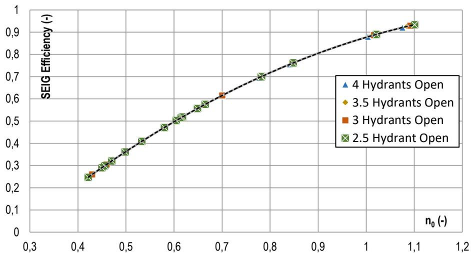
Figure 25 - SEIG (electrical) efficiency by relative imposed rotational speed
