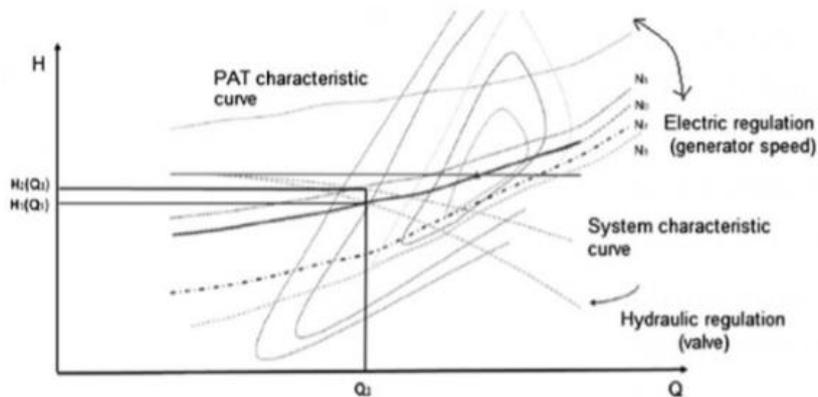
Figure 15 - Hydraulic and Electric Regulation (HR/ER/HER) in a hill diagram [62]
