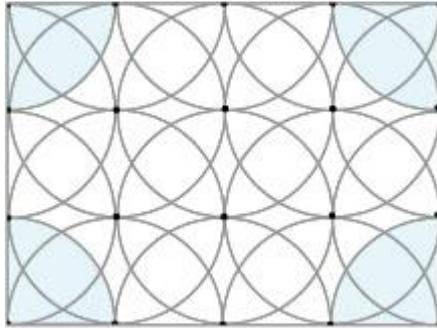
Figure 11 - Irrigation Sprinklers coverage area [57]
