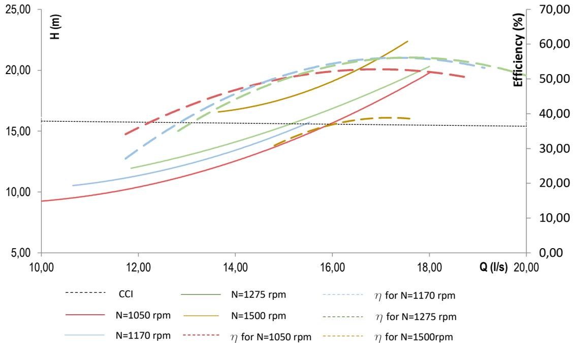
Figure 41 - PAT 2 operating conditions for different rotational speed - Head/Flow/Efficiency analysis
