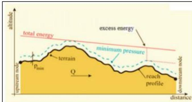
Figure 12 - Available energy which can be extracted in a pipe system [62]
