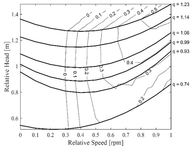
Figure 30 - Relative head, flow, rotational speed and global efficiency
