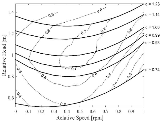
Figure 29 - Relative head, flow, rotational speed and PAT efficiency
