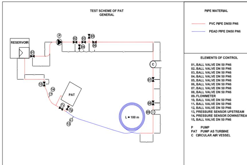
Figure 19 - PAT pilot station scheme
