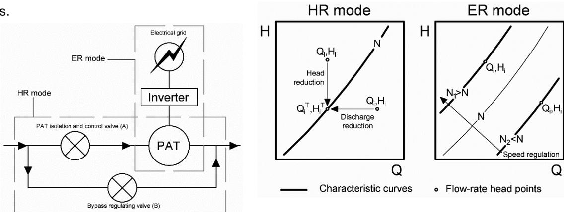
Figure 14 - Hydraulic or Electric Regulations (HR/ER) PAT installation scheme and operating conditions [66]
