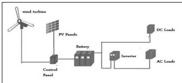
Figure 16 - (PV + WT) Hybrid power system [68]
