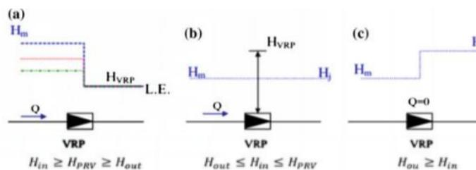
Figure 13 -PRV behaviour: a) Active, b) Passive open, c) Passive closed [63]
