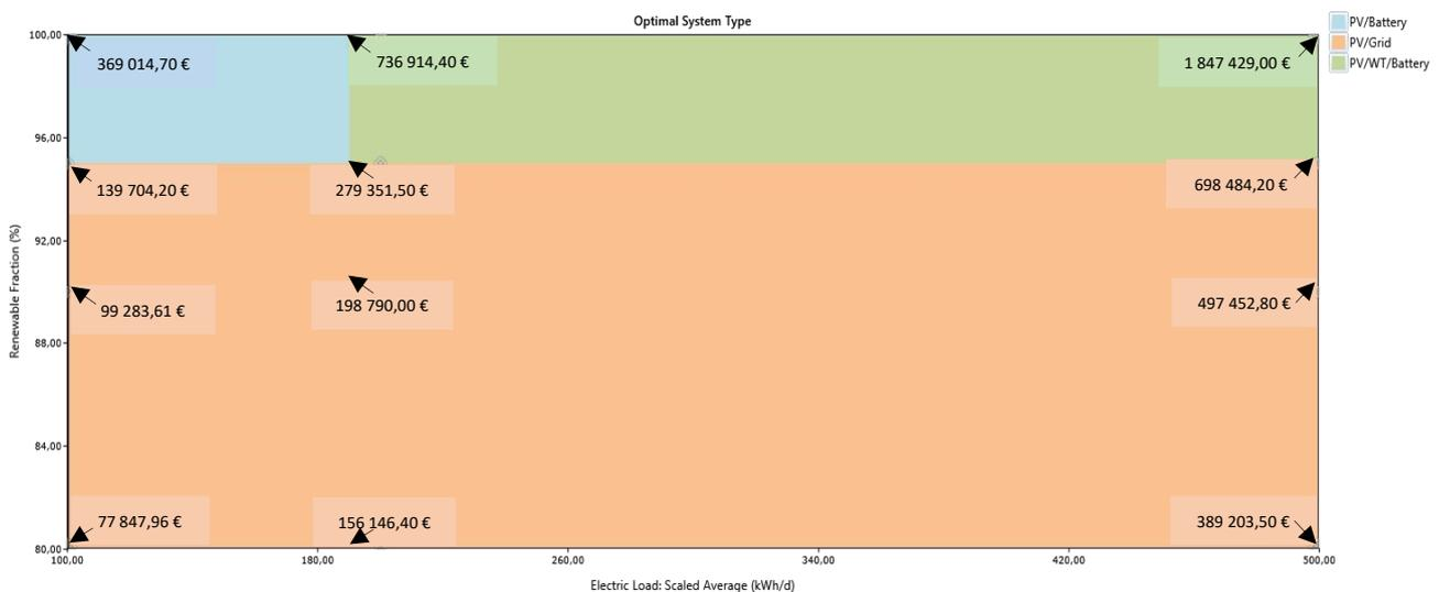
Figure 45 – Optimized system configuration for a sensitivity analysis based on the renewable percentage and the electric load
