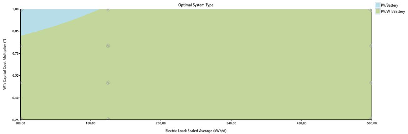
Figure 46 - Off-grid (100% renewable) optimized system configuration for different electric needs and WT cost multiplier values
