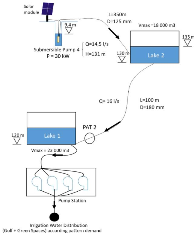
Figure 40 - High Region of BCC WDS - PAT 2 scenario schematic design.
