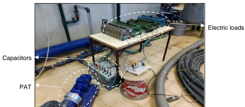
Figure 23 - Electrical components of the PAT Pilot Station
