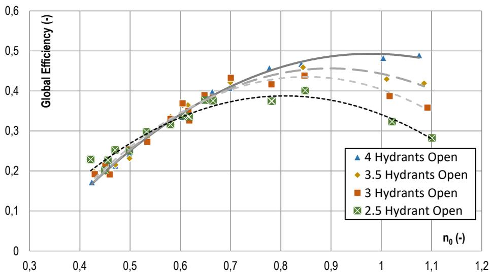
Figure 27 - Global efficiency by relative imposed nominal rotation for different flows
