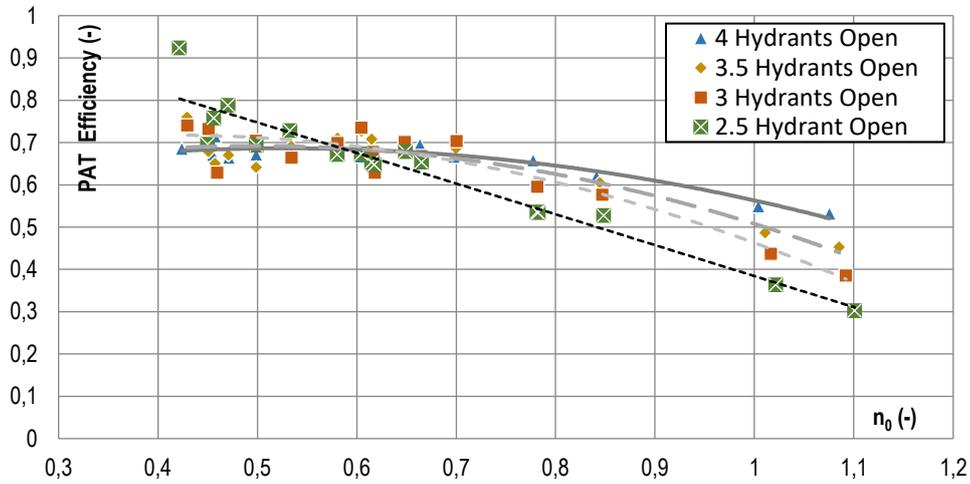
Figure 28 - PAT efficiency by imposed nominal rotation for different flows
