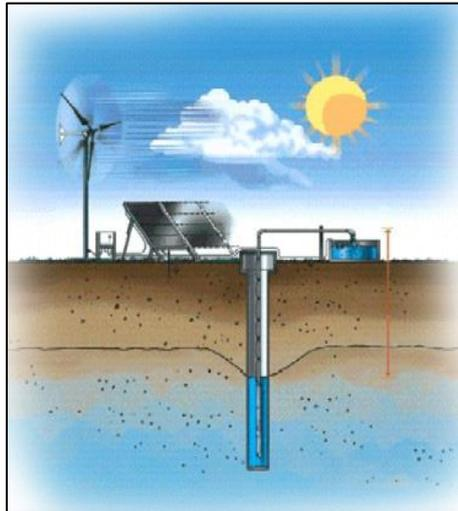
*Figure 17 - Hybrid pump system scheme [70]*
