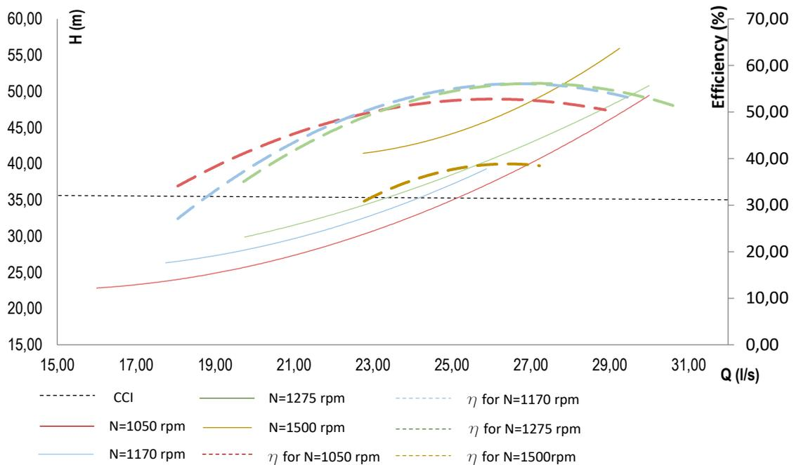
Figure 39 - PAT 1 operating conditions for different rotational speed - Head/Flow/Efficiency analysis
