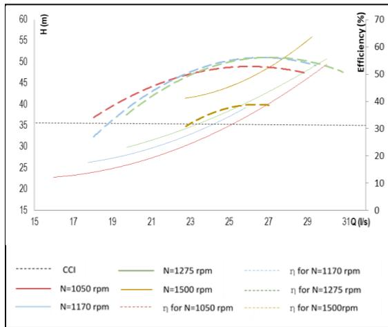
**Figure 11 - PAT 1 operating conditions for different rotational speed - Head/Flow/Efficiency analysis**
