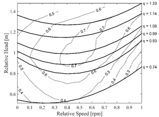
Figure 3 - Relative head, flow, rotational speed and PAT efficiency
