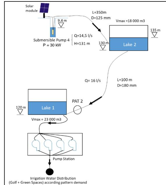
**Figure 12 - High Region of BCC WDS - PAT 2 scenario schematic design**
