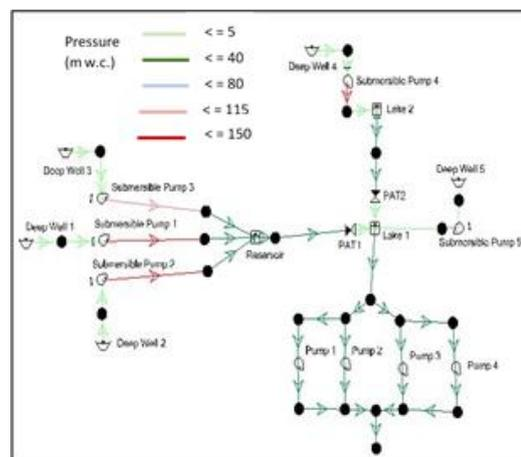
Figure 8 - Pressure in the network at 07:00
