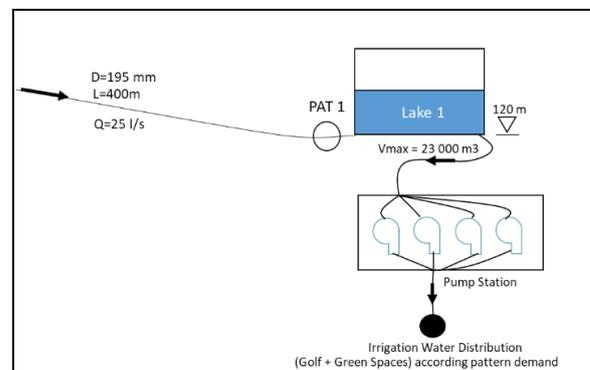
Figure 10b - Medium Region of BCC WDS – Reservoir tank to Storage Lake
