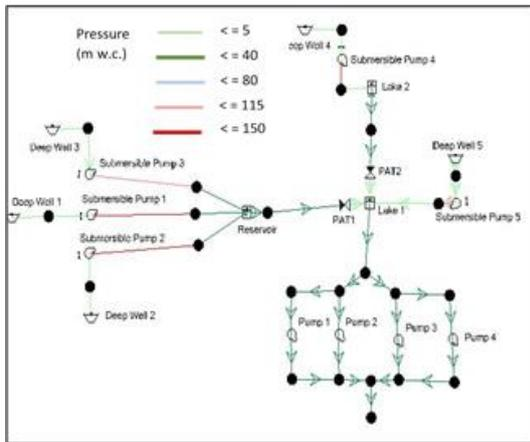
Figure 9 - Pressure in the network at 17:00
