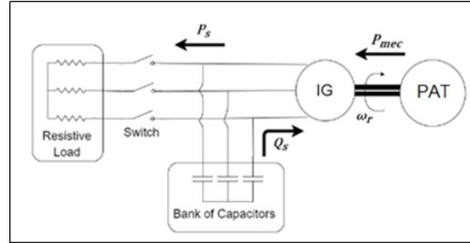
Figure 2 - Off-grid PAT electrical connection
