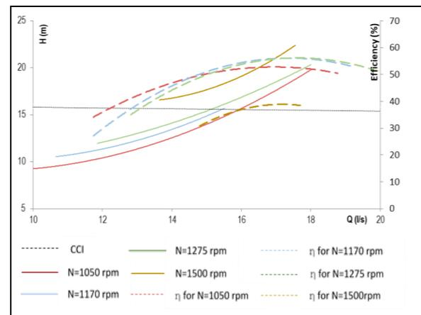
**Figure 13 - PAT 2 operating conditions for different rotational speed - Head/Flow/Efficiency analysis**
