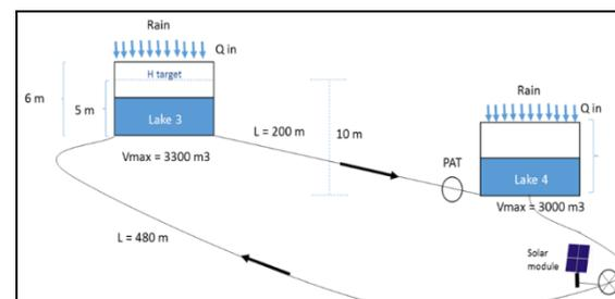
**Figure 14 - Scheme of the SUDS in BCC (Low Region of BCC)**
