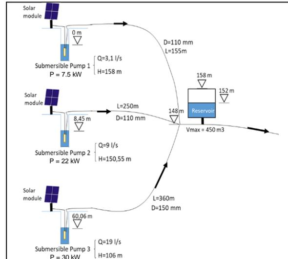
Figure 10a - Medium Region of BCC WDS – Submersible Pumps to Reservoir tank
