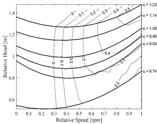
**Figure 4 - Relative head, flow, rotational speed and global efficiency**
