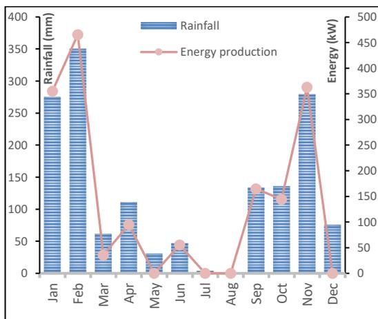
**Figure 15 - Energy production for the year 2014 based on a SUDS and PAT technology**
