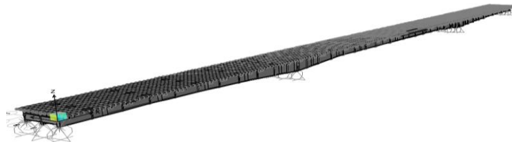
Figure 5.1 - Finite element model of the deck (image, CSI SAP2000)
