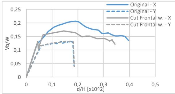
Figure 3.9 – Capacity curves for the original model and the removed frontal walls model
