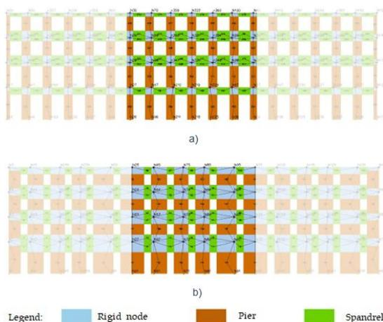
Figure 3.2 - Macro-elements mesh for the modelled building
