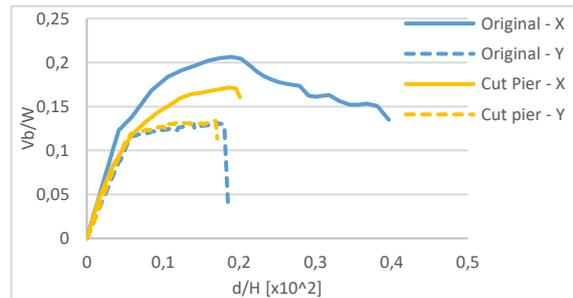
Figure 3.7 – Capacity curves for the original model and the cut of a pier model
