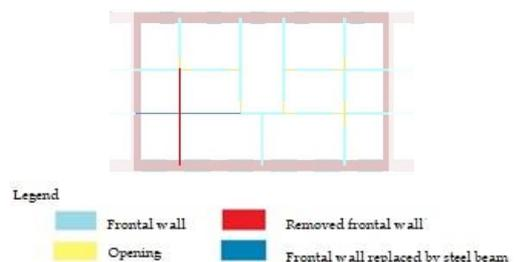
Figure 3.8 – Structural modifications on the upper floors
