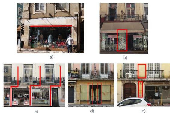
Figure 4.5 – Types of discontinuities for ground floor piers
