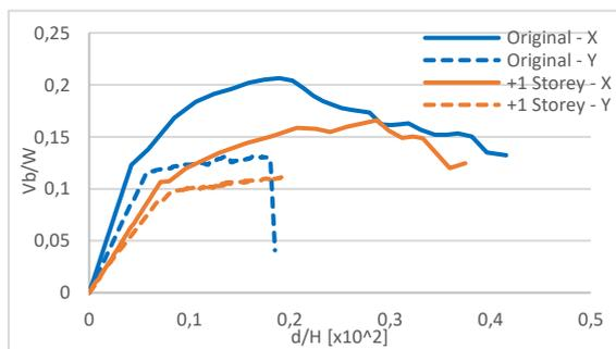
Figure 3.5 - Capacity curves for the original model and the increasing storey model
