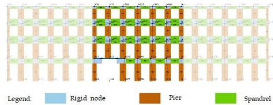
Figure 3.6 – Front façade mesh after cutting a pier
