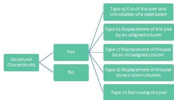
Figure 4.4 – Classification of the ground floor piers
