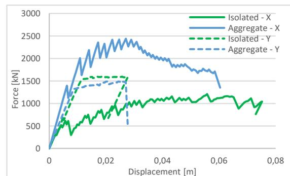
Figure 3.3 - Capacity curves for the isolated building model and the building inserted in aggregate model
