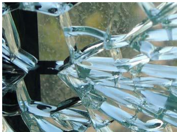
Figure 4.4: NiS (Nickel Sulphide) inclusions cause “spontaneous” glass breakage [11]
