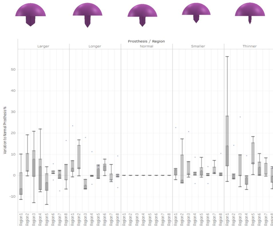
Figure 11 - Average relative difference in strain energy density (%) between the standard and modified models for the flexion load case. The x-axis represents, on top, the prostheses modeled and, on bottom, the eight regions of the humerus defined.
