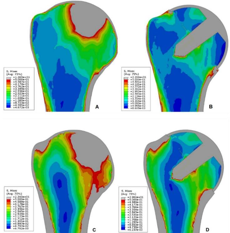
Figure 6 - Von Mises stress (MPa) distribution in the intact bone (A) and in the implanted bone with the Normal Prosthesis (B) for the flexion load case and in the intact bone (C) and in the implanted bone with the Normal Prosthesis (D) for the abduction load case.
