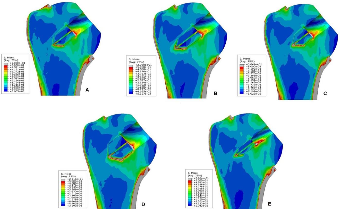
Figure 7 - Von Mises stress (GPa) distribution in the bone implanted with the Normal Prosthesis (A), the Longer Prosthesis (B), the Smaller Prosthesis (C), the Larger Prosthesis (D) and the Thinner Prosthesis (E) for a Flexion movement.
