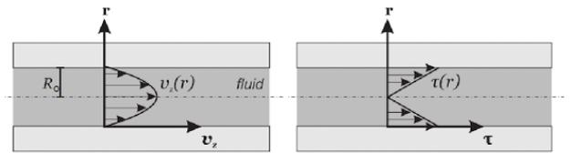
**Fig. 7** Schematic of a laminar flow with a parabolic profile due to shear stress felt near the borders of the channel [54].
