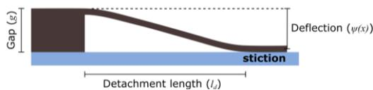
**Fig. 6** Cantilever under stiction effect [13]. The beam is permanently stuck to the substrate.
