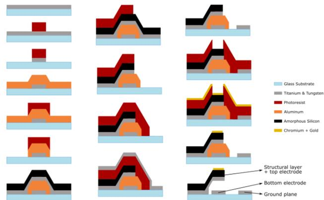
Fig. 9 Schematics of the entire process of MEMS micromachining.
