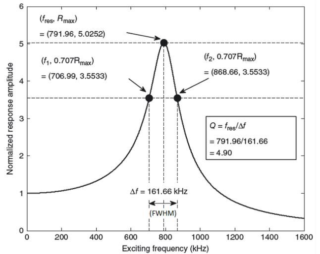
**Fig. 4** Example of a resonance peak of a cantilever with the calculation of the  $Q$  factor [40].
