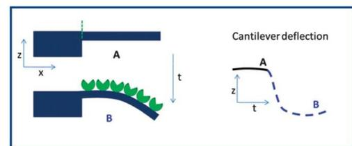
Fig. 2 Cantilever operating in the static mode [3]. In this case, the monitored parameter is the tip deflection.
