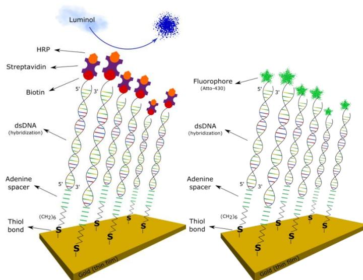
**Fig. 8** Schematics of the two techniques employed for target detection: (*left*) chemiluminescence and (*right*) fluorescence.
