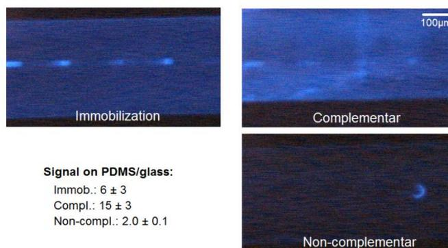
**Fig. 11** Results obtained for immobilization and hybridization. (*left*) A plot of the signal on top of Au surfaces is presented along with the (*right*) images captured by chemiluminescence. The bright rectangles correspond to the Au patterns.
