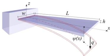
Fig. 1 Schematics of a cantilever.
