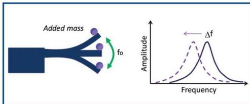
**Fig. 3** Cantilever operating in the dynamic mode [3]. Mass is measured by shifts in the resonance frequency.
