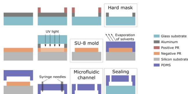
Fig. 10 Schematics of microfluidics fabrication.
