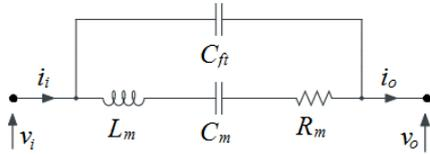
**Fig. 5** Butterworth-van-Dyke model for a resonator with parasitic capacitance.  $C_{ft}$  is the feed-through capacitance while  $L_m$ ,  $C_m$  and  $R_m$  are the electrical equivalents of the mechanical model.
