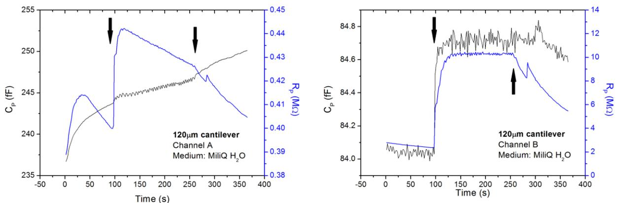
**Fig. 13** Results obtained with the capacitive readout setup for two cantilevers with 120µm length placed in two different channels. The black arrows are pointing the instants in which the pump was turned on and off.
