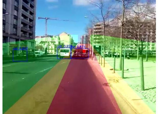
Fig. 1. Risk assessment framework: The estimation of the Focus of Expansion (red point) allows a representation of different level risk areas in the image. Risk is evaluated taking into account the objects in the image (blue rectangles) and the path of the cyclist (red area in the image).
