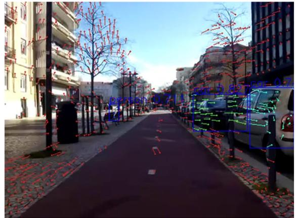
Fig. 3. Object associated weights given the confidence score outputted by the NN. Red vectors correspond to  $s_k = 0$ , blue vectors  $s_k = 0.711$ , cyan vectors  $s_k = 0.741$ , and green vectors to  $s_k = 0.827$ .
