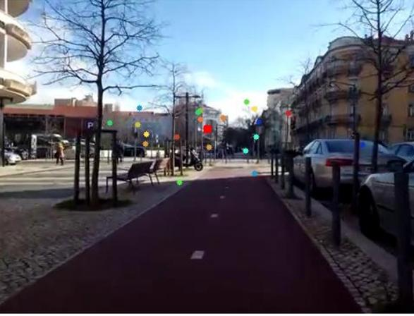
Fig. 5. The weighted average of the previous and current FOE (small colored points) and the result of this operation (large red point in the center of the image).
