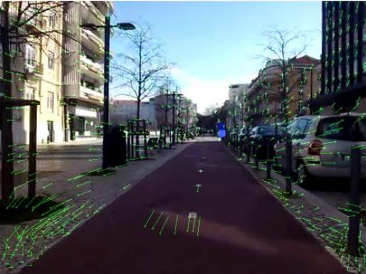
Fig. 8. Example of the FOE estimation using the Huber Loss Distance optimization. The light blue point represents the solution without any weight consideration, whereas the dark blue point represents the optimization using weights.
