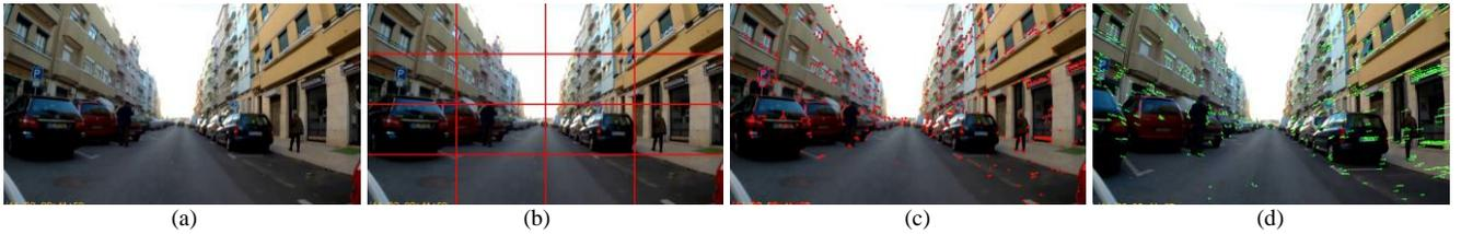
Fig. 7. Procedure to compute the optical flow: given a frame (a), divide it in 16 (b), apply the CLAHE filter to each and calculate the Shi-Tomasi feature detection (c) and finally compute the optical flow to the previous frame (d).
