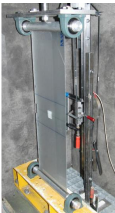
Figure 23 – Buckling test setup (source: Spitzhüttl et al. , 2014)
