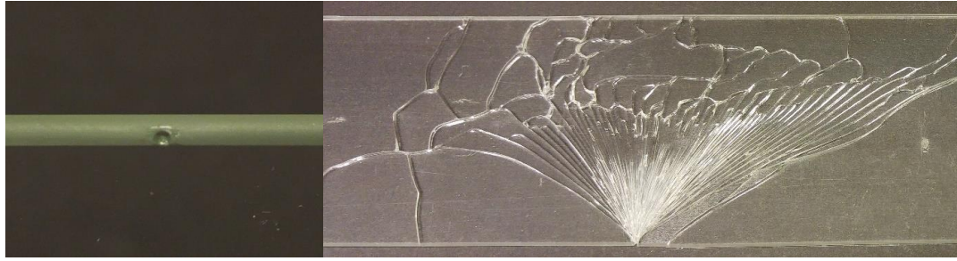
Figure 48 – Detail of a flaw on the edge of the sample (left tested and corresponding cracking pattern (right))
