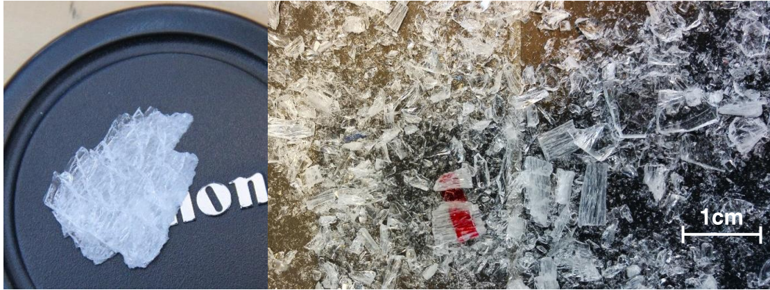
Figure 84 – Shatters after breakage of glass: detail with a 6cm diameter lens cover and with a 1cm strain gauge
