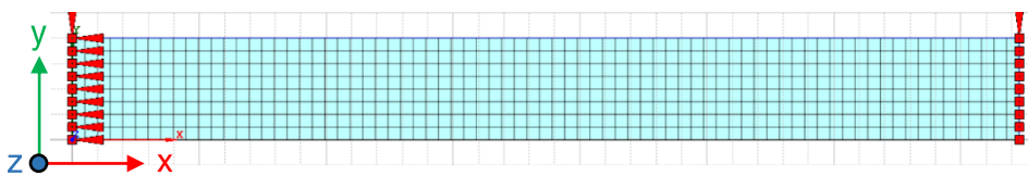
Figure 85 – Geometry, mesh and boundary conditions for the buckling model
