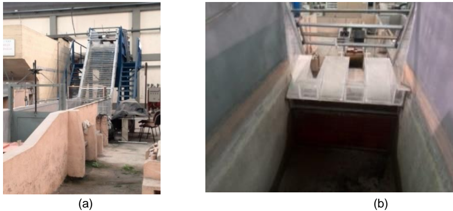
Figure 2 – Experimental set-up: (a) general downstream view; (b) upstream view of the PKW.
