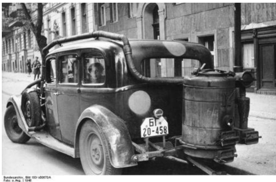
Fig. 16 Car powered with gas generator [50]
