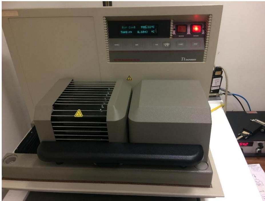
Fig. 19 TA Instruments SDT 2960 Simultaneous DSC-TGA
