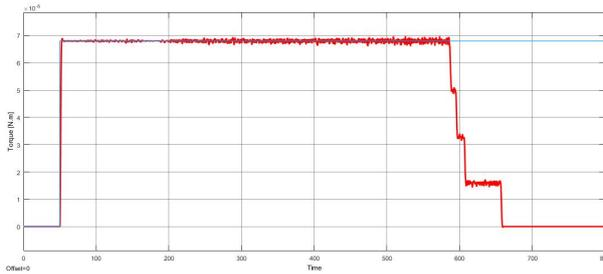
Figure 10: Torque generated in the Y-axis direction by the overall RWS w.r.t. the satellite's body-fixed reference frame in normal conditions until saturation
