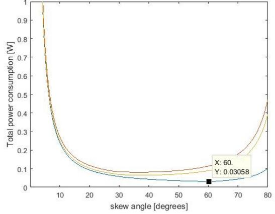
Figure 6: RWS power neglecting the electronics power consumption as function of the skew angle. ( $\beta_1 = 45 \text{ deg}$  in blue;  $\beta_1 = 40 \text{ deg}$  in green;  $\beta_1 = 30 \text{ deg}$  in red). Minimum power consumption for  $\beta_1 = 45 \text{ deg}$  and  $\beta_2 = 60 \text{ deg}$
