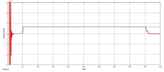
Figure 11: Torque generated in the Y-axis direction by the overall RWS w.r.t the satellite's body-fixed reference frame assuming wheel #1 has failed until saturation
