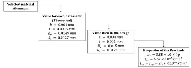
Figure 4: Optimal solution design for the flywheel using aluminium
