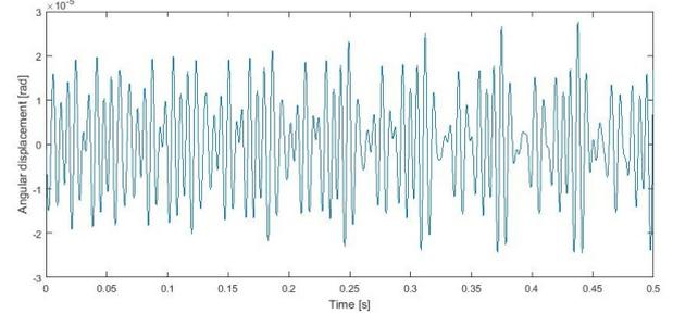
Figure 8: Angular displacement of the satellite around the  $y$ -axis w.r.t. the satellite body-fixed reference frame
