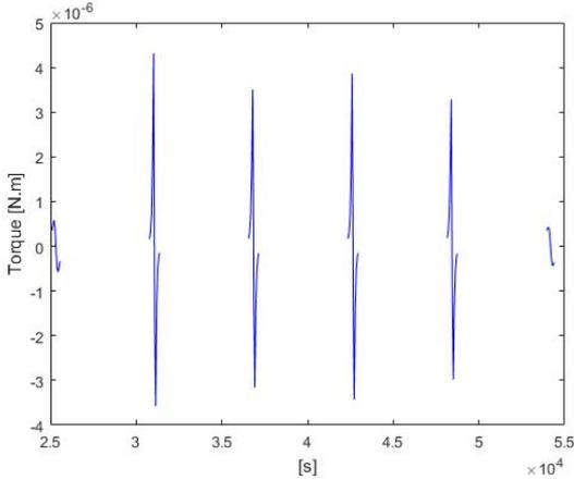
Figure 1: Torque that should be applied on ECOSat-III during its crossing above Victoria (maximum angular rate), considering the absence of external perturbation torques
