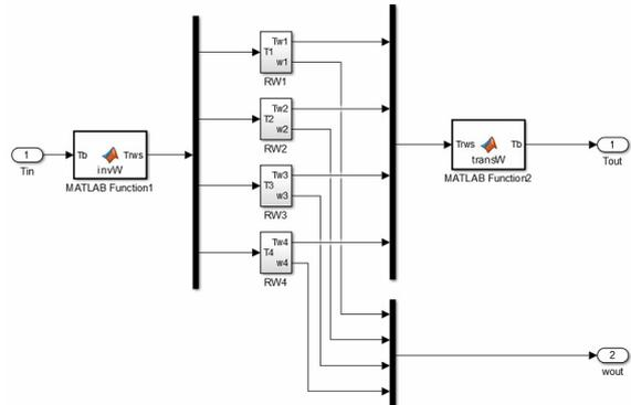
Figure 9: Overall RWS simulink block
