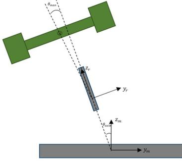
Figure 7: Deflection angles representation due to internal disturbance torques sources in the Reaction Wheel
