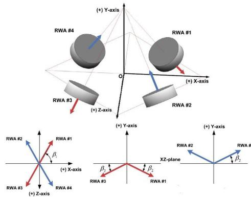
Figure 5: Pyramid configuration [15]
