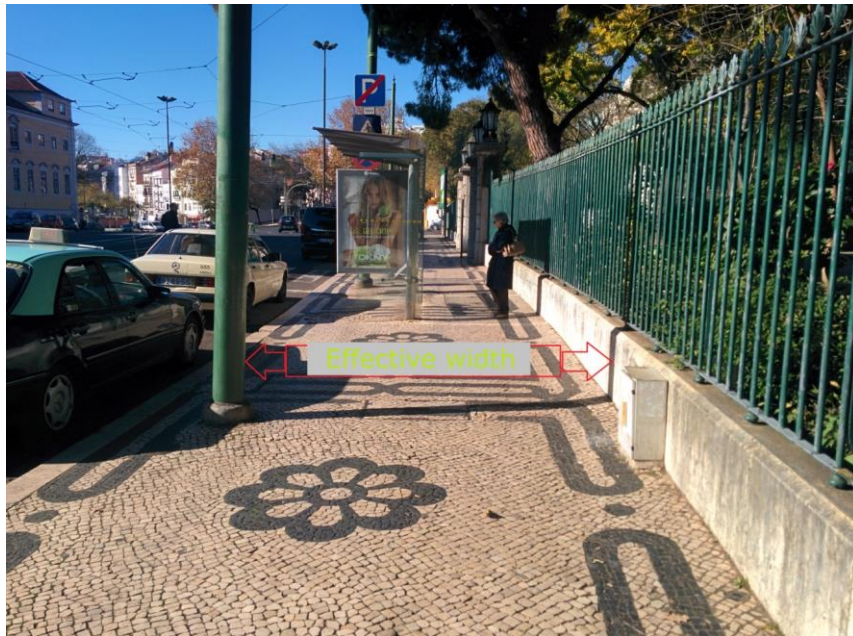
Figure 49- Measuring effective width
