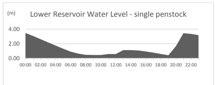
Figure 28 - Results for hourly water level of the lower reservoir for one scenario simulation of single penstock
