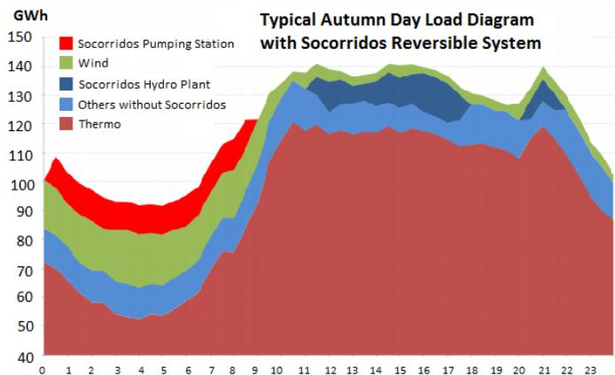
Figure 13 – Load diagram in grid with Socorridos Reversible System (adapted from (EEM, 2010))
