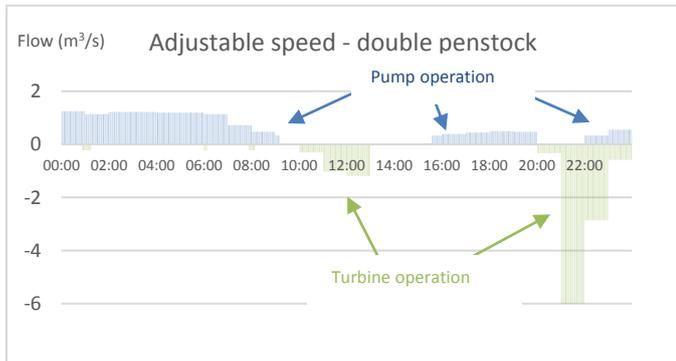
Figure 30 - Results for one scenario simulation of adjustable speed with double penstock
