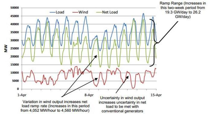
Figure 7 – Impact on net load from increased use of variable generation units (Denholm et. al, 2010)
