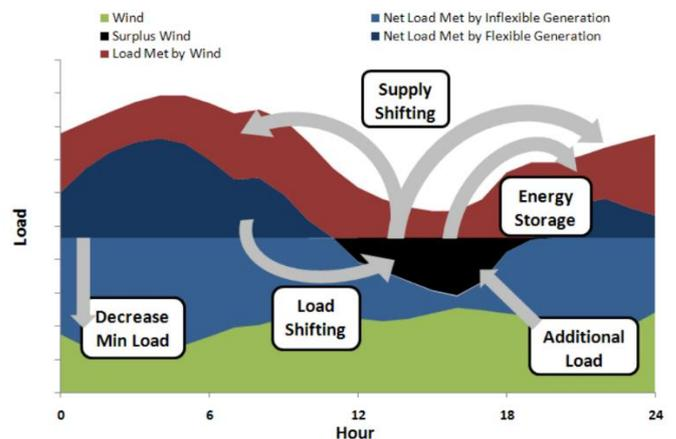
Figure 9 – Storage as an option for increasing the use of variable RES by decreasing curtailment (Denholm et. al, 2010)
