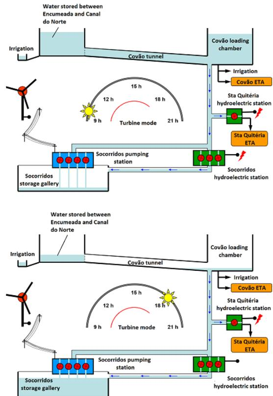
Figure 10- Snapshots of the schematic operation of the system in turbine mode (adapted from (EEM, 2006))
