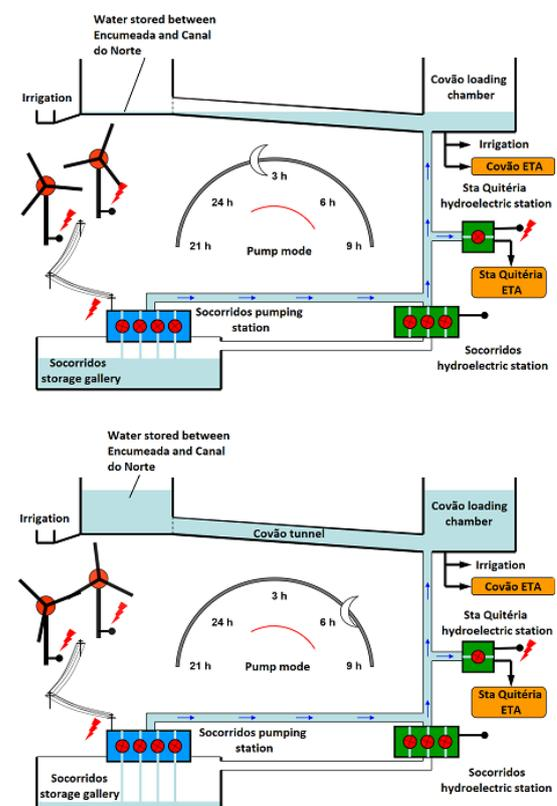
Figure 11- Snapshots of the schematic operation of the system in pump mode (adapted from (EEM, 2006))
