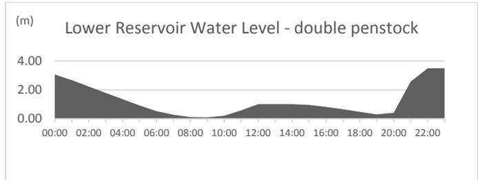
Figure 33 - Results for hourly water level of the lower reservoir for one scenario simulation of double speed
