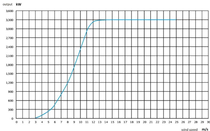
Figure 16 – VESTAS V90 wind turbine power curve
