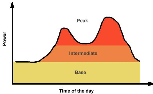
Figure 1 - Daily load curve separated into base, intermediate and peak load (adapted from Cordaro (2008))
