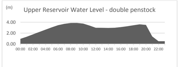
Figure 32 - Results for hourly water level of the upper reservoir for one scenario simulation of double speed
