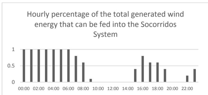
Figure 17 - Hourly percentage of the total generated wind energy that can be fed into the Socorridos System
