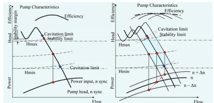
Figure 4- Operating ranges of fixed-speed (left) and adjustable-speed pumps (adapted from Krenn et al (2013)).
