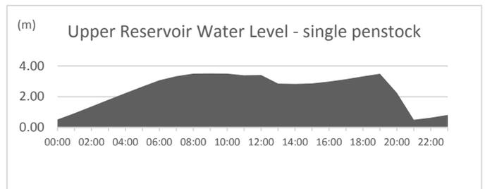
Figure 27 - Results for water level of the upper reservoir for one scenario simulation of single penstock
