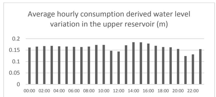
Figure 19 –Average hourly consumption derived water level variation in the upper reservoir (m)
