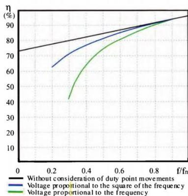
Figure 22 – Operating efficiency of VFD (FLYGT, 2011)
