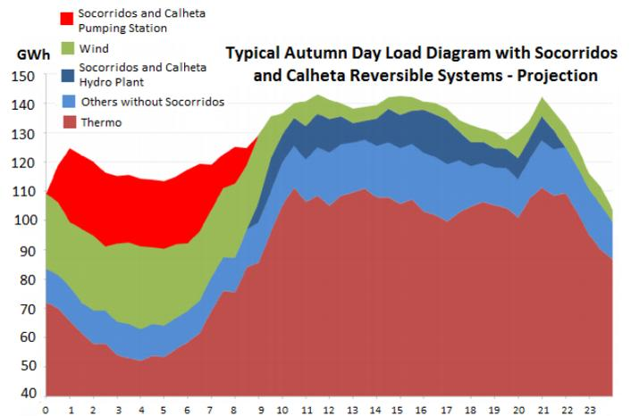
Figure 14 - Load diagram in grid with both Socorridos and Calheta Reversible System (adapted from EEM, 2010)
