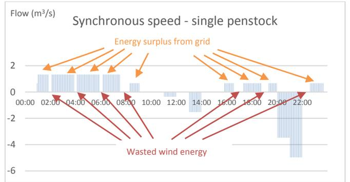
Figure 26 - Results for one scenario simulation of synchronous speed with a single penstock
