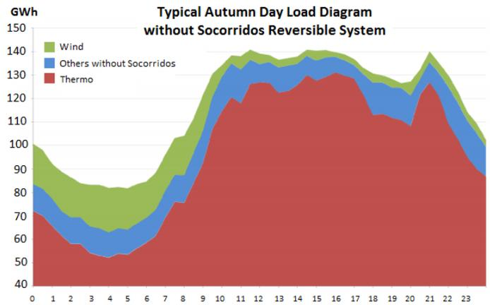
Figure 12– Load diagram in grid without Socorridos Reversible System (adapted from (EEM, 2010))
