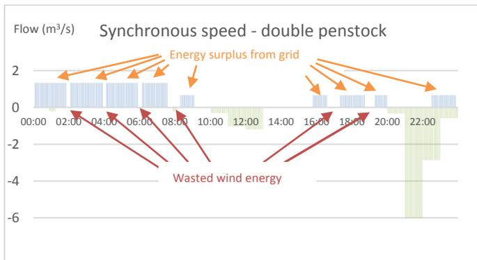
Figure 31 - Results for one scenario simulation of synchronous speed with double penstock
