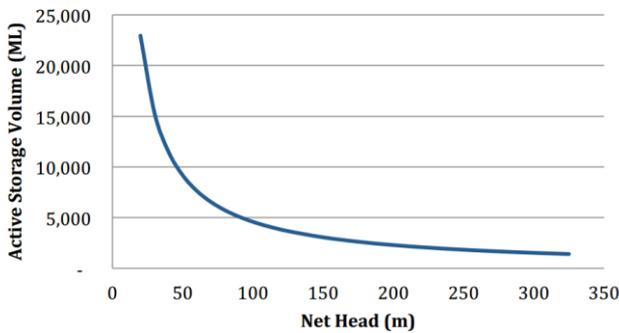
Figure 3 - Relationship between water volume requirements as a function of net head between reservoirs, for 1,000 MWh of stored energy (Hearps et al., 2014)
