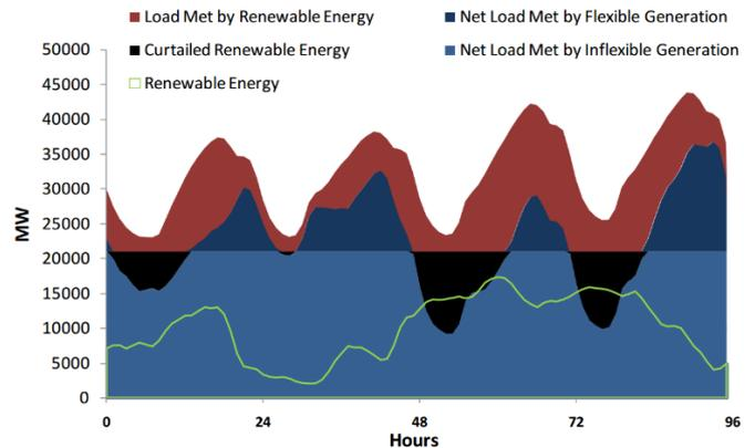
Figure 8 – Variable RES generation curtailment in a high RES penetration grid (adapted from (Denholm et. al, 2010))
