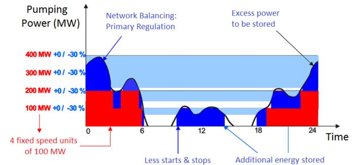
Figure 5 - System reserve and power storage from variable-speed vs single-speed pumped storage (Ciocan et al, 2012)
