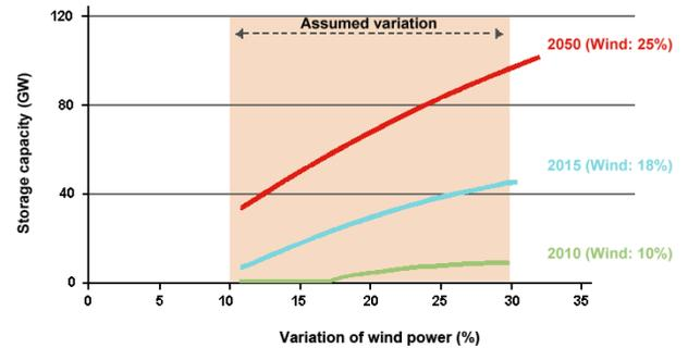
Figure 2 - The relationship of net wind power variation and necessary storage capacities (adapted from (Inage, 2009))
