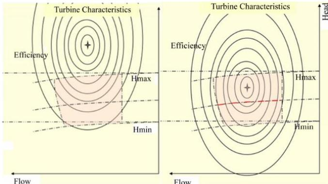
Figure 6 - Operating ranges of fixed-speed (left) and adjustable-speed (right) turbines (adapted from Krenn et. al (2013))
